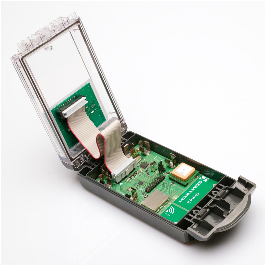
Figure 3-1: Mote II with open Cover
